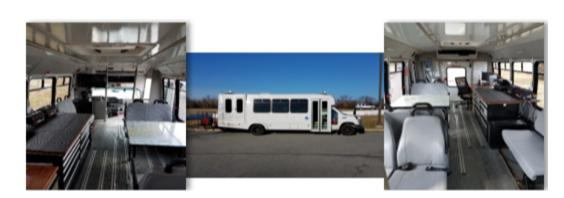
DelDOT has equipped a "Drone Bus" that functions as a mobile traffic management center (TMC) when the UAV is in long-operation use. The drones/UAVs are used to enhance situational awareness, conduct debris assessments, assess traffic mitigation, conduct bridge inspections, archeological inspections and dune erosion analyses.
