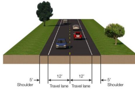
Figure 6. Typical Two-Lane Undivided Roadway Section for Parallel Corridors
