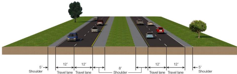
Figure 4. Typical Four-Lane Divided Roadway Section for Parallel Corridors
