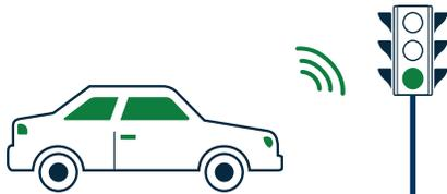
**Vehicle to Infrastructure:** The traffic signal ‘talks’ to the vehicle and offers information about the traffic signal timing, potential pedestrians present, and other location specific information. For example, the traffic signal may tell you that the light is about to turn green or that a pedestrian has requested to cross.
