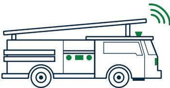
**Emergency Vehicle Preemption (EVP):** The emergency vehicles “talk” to the traffic signals which adjusts signal timings to clear traffic in the direction of travel before the emergency vehicle reaches the intersection. Providing faster response times and safer travel for all motorists.
