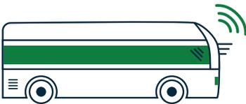
**Transit Signal Priority (TSP):** The transit vehicle “talks” to the traffic signal to ask if the traffic signal can provide additional green time for the transit vehicle to progress through the signal. Providing more efficient and reliable transit services.
