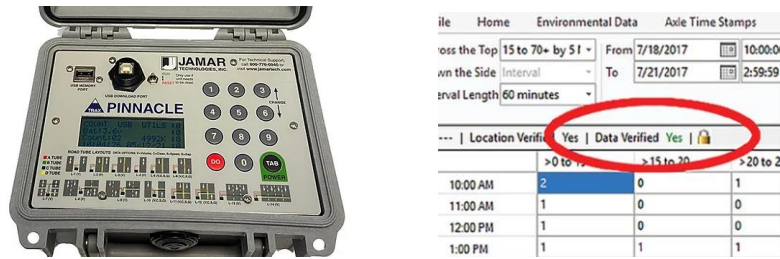
Figure 7: JAMAR TRAX Pinnacle counter and data verification software.
