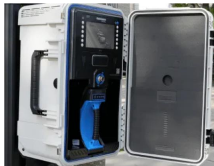
Figure 9: Miovision Scout Plus video-based counter.
