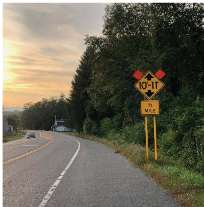
Figure 23. Low-clearance advance warning sign. (Source: VHB)
