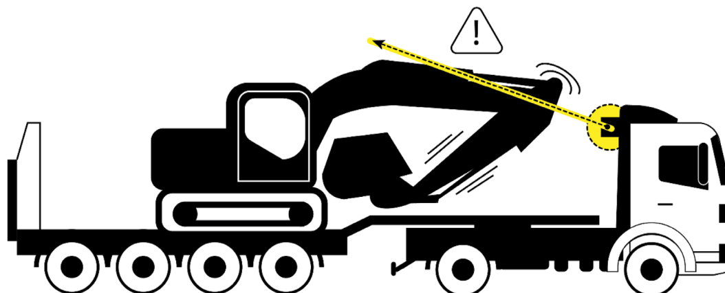
Figure 46. Overheight detection and driver warning system example (Source: VHB).
